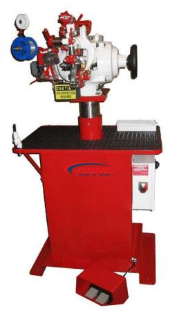
Smoother performance Eliminates brake & clutch Lower maintenance costs Fewer adjustments Available with or without pincers Head height easily adjusts to operator Accepts 5# or 65# staple wire rolls Easy adjustment for staple length
